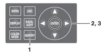
1. When the MEAS screen is displayed, press MEMORY key to switch to the MEMORY screen.
